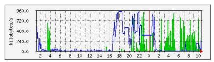
The difference between the first and second step is very obvious here. While there were only write operations while splitting the MPEGs into images (blue), they were read again for rendering the videos in the second step (green). While the first step was still running between 9pm and 11pm, the second step was running in parallel for rendering the speedskaters' videos.
